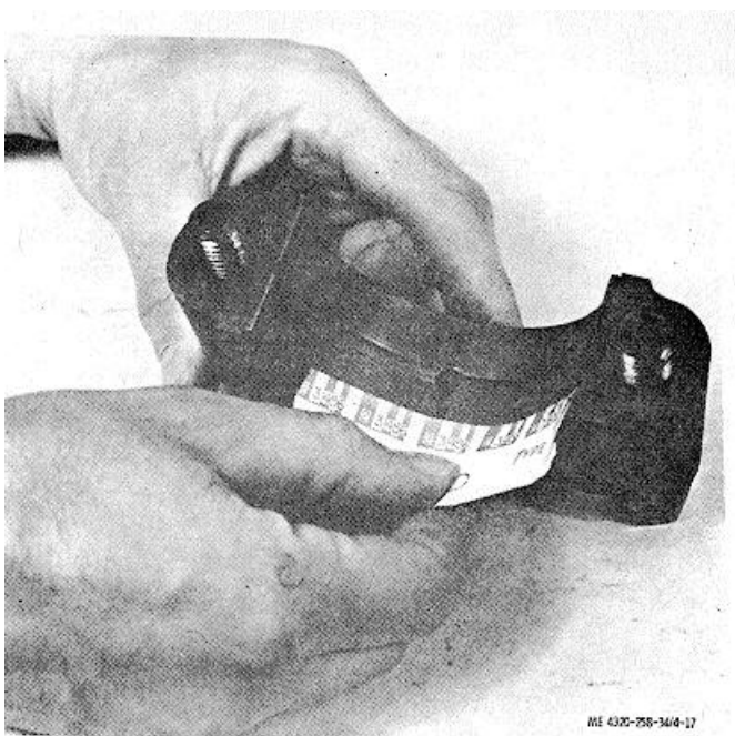
Figure 4-17. Checking bearing clearance with plastigage.
